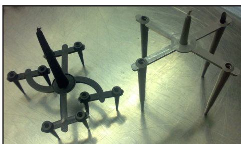
An oversized 3-plate cold runner results in higher production costs.
